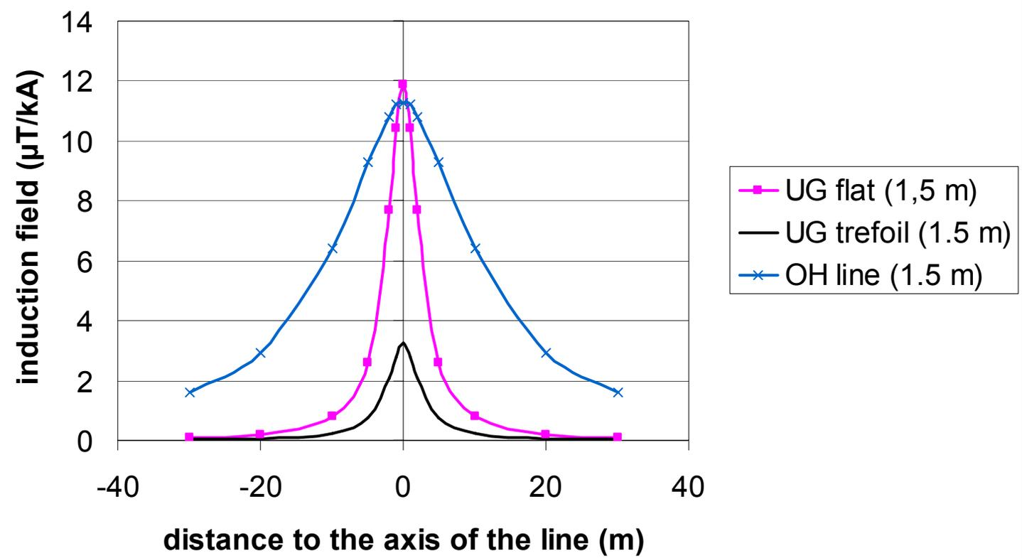
Typical field levels at 1.5 m above ground for a 400 kV overhead line compared with a 400 kV underground cable
